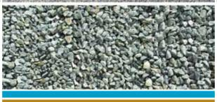
6 inch depth of well compacted non-frost susceptible sub base material installed in compliance with DOT specifications
